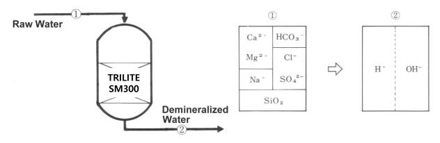
TRILITE SM300 can produce high purity water through the above mechanism, applied to post RO/EDI. It features high anion conversion rate and specific gravity and excellent SiO<sub>2</sub> removal capacity.
